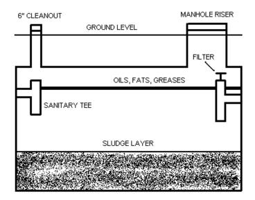
The sewer line from the house to the tank must be a minimum of SDR 35 with a cleanout located between the house and the tank. The lines must have a slope of one 1/8" per foot to the tank and to the trenches. The line into and out of the tank must be schedule 40 for at least ten feet.
