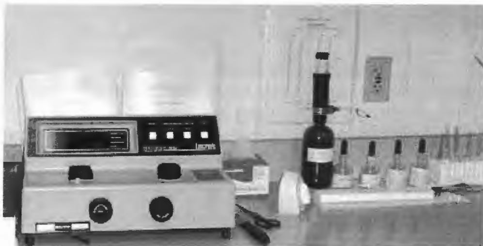
Figure 4. Methylene blue testing station, with test tubes, testing solutions, and equipment.
