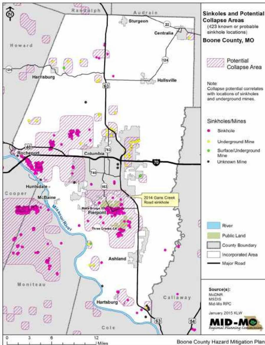
The potential for collapse from underground mining is primarily in the northern part of Boone County and associated with coal fields (Figure 3.27). Prior to larger open pit mining activities in Boone County, there were numerous “Mom and Pop” underground coal mining operations; these were small mines using a series of tunnels and pillars. There are 200 known mining locations in the planning area.
