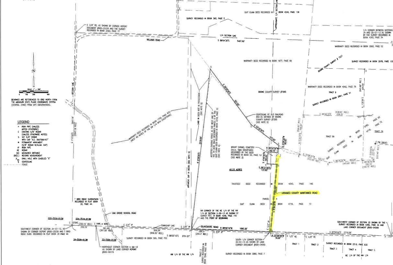
BEARINGS ARE REFERENCED TO GRID NORTH FROM THE MISSOURI STATE PLANE COORDINATE SYSTEM (CENTRAL ZONE) FROM GPS OBSERVATIONS.
