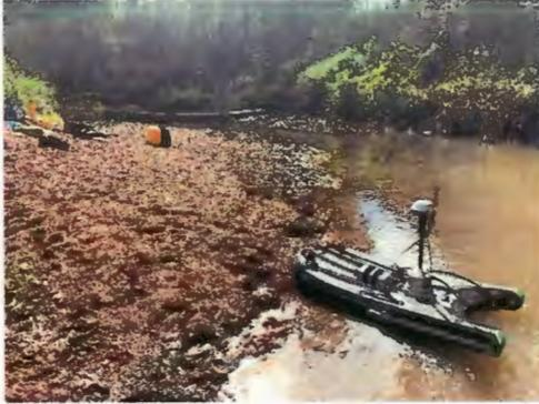
*Geosyntec collecting a stream discharge measurement using a Sontek RiverSurveyor M9 acoustic doppler current profiler with hydroboard and RTK base station.*
