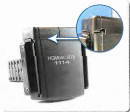
**Figure 27. Physical Evidence of Tamper**
