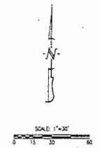
BEARINGS ARE REFERENCED TO GRID NORTH OF THE MISSOURI STATE PLANE COORDINATE SYSTEM (CENTRAL ZONE), DETERMINED FROM GPS OBSERVATION.
