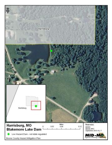
A more detailed mapping of the area of Blakemore Lake Dam on the southeastern edge of the village of Harrisburg shows that the dam is actually located outside the city limits (Figure 4.35). If a dam failure occurred, the drainage from this dam would move away from the village so the dam is not considered a threat to Harrisburg.
