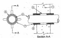
Wall Assembly — Min 7-5/8 in. thick reinforced lightweight or normal weight (100-150 pcf) concrete wall assembly. Wall may also be con-structed of any UL Classified Concrete Blocks\*. Max diam of opening
