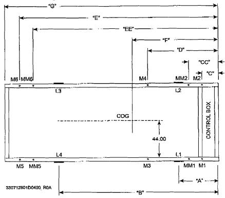
NOTE: "L" are lifting tab locations, "M" are standard isolator locations, MM and M3 and M4 are for seismic mounts.
